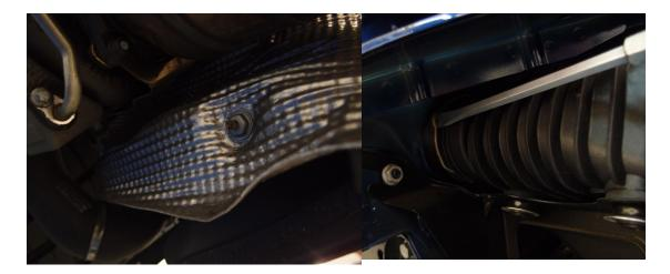
On the underside of the vehicle, where the turbo compressor outlet meets the other intercooler hose, you need to loosen the 7mm hose clamp bolt and pull the hose off from the compressor.
