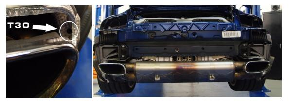
Step 3 – Remove Intercooler & Catalytic Converter
