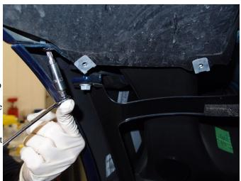
Underneath the car, there are 3x T30s on each side (6x total) that need to be removed.
