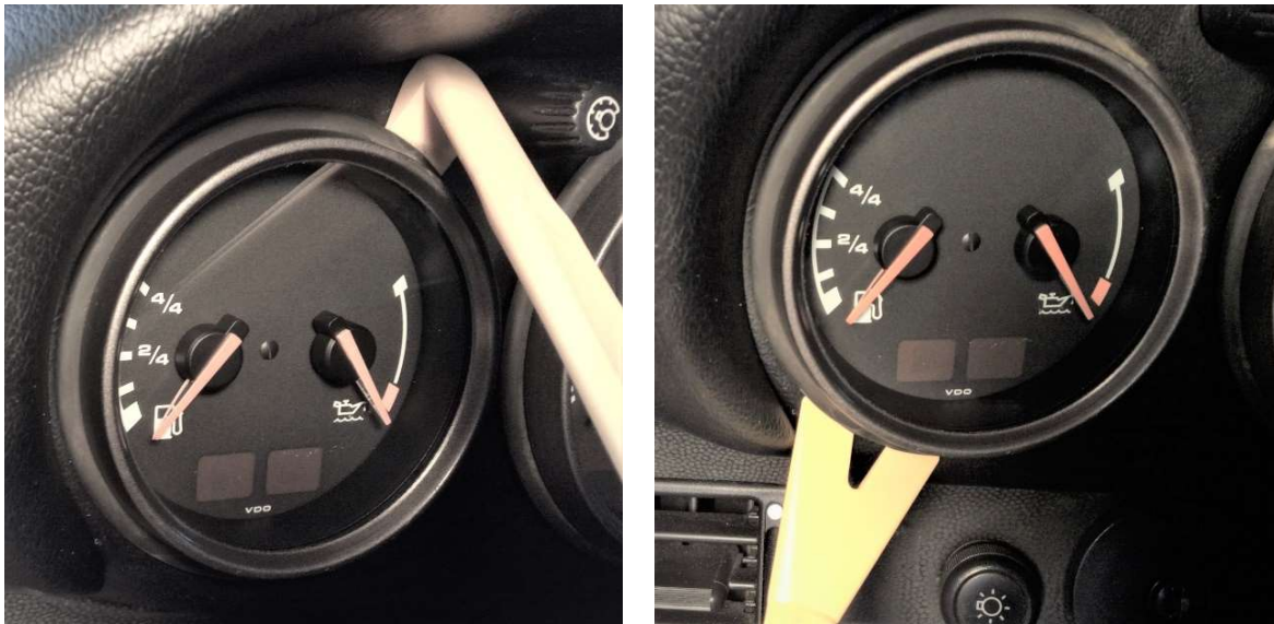
Figure 1 Use plastic pry bars to loosen gauge
